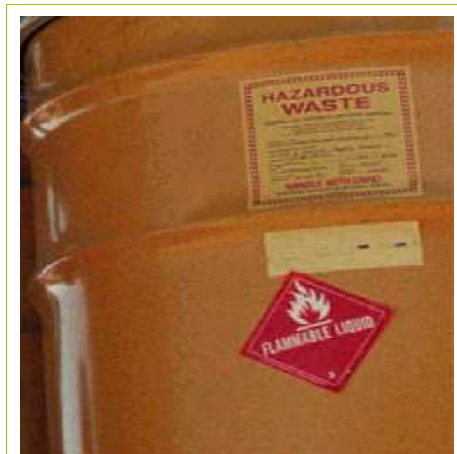
Figure 5: Labels on a hazardous waste containing drum indicating waste type and associated hazard
